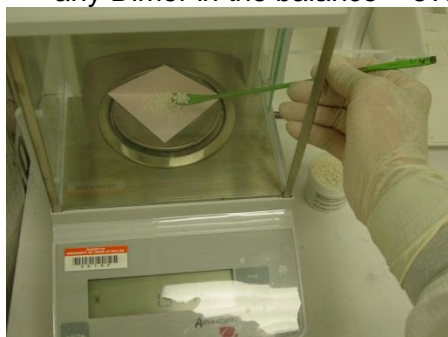
Figure 8. Weigh out the desired mass of Parylene Dimer onto a weighing paper or Al Boat.
