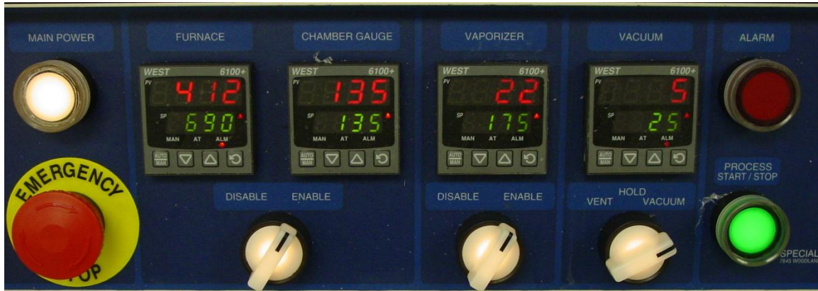
Figure 1A. Parylene Deposition tool front panel.
