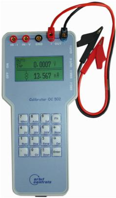
The instrument is supplied from internal battery and permits an uninterrupted operation of 3-4 hours with the output current between 0 and 20mA. For higher output currents up to 100mA the calibrator has to be connected to the charger. When the display shows BAT of the battery capacity, the calibrator has to be connected to the charger.
