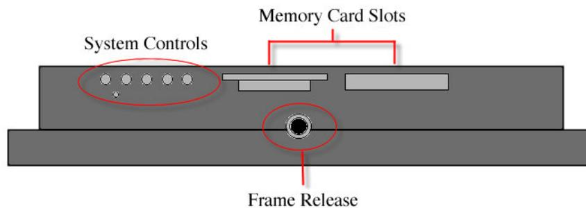
Two slots for CF, SM, MS, MSPRO, SD, MMC, IBM MICRODRIVE: 7 types of memory card ports.
