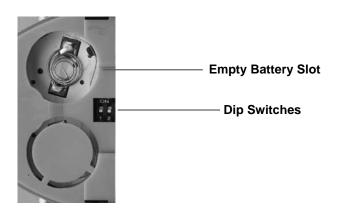
The DIP Switches above are used to set the IR Channel. Changing channels will alleviate issues that may occur if the unit or remote control responds or interferes with other non-Gefen equipment. This setting must match the IR Channel setting on the unit. Please see page 18 for setting up the IR Channel on the unit.
