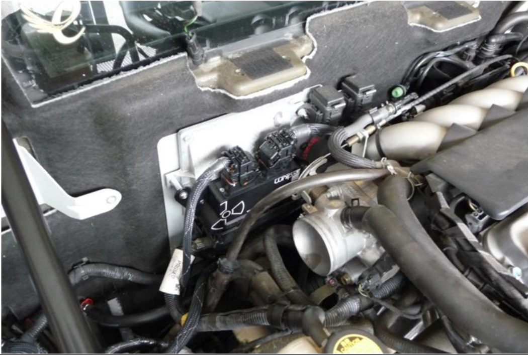
9. Engine side of the main harness installed.
