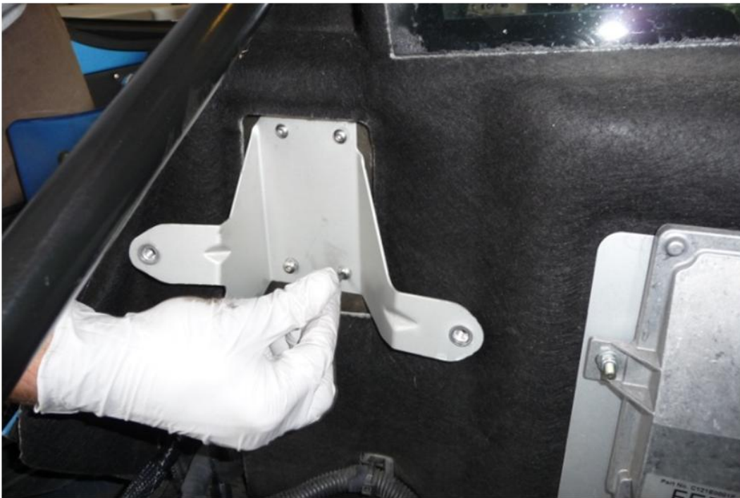
10. Remove the air intake system and drill out the six rivets holding the air box bracket to the bulkhead wall. Four rivets are located on the vertical face (shown) and two are located on the top face hidden by the carpet. Insert the included M5 button head Allen screws into the holes as place holders until the EMS bracket is installed inside at a later step.
