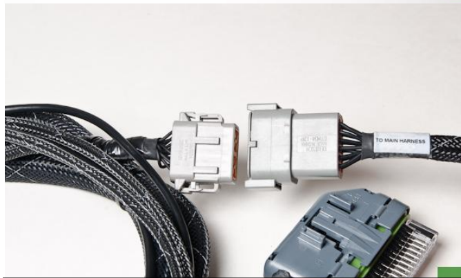
The auxiliary harness attaches to the main harness.
