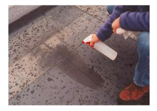
**Note:** Prior to using the Air-Sure Test Solution, ensure that the Test Solution has not passed its expiry date, and is functioning as intended. The solution should be tested on a 'known' leak; if the solution does not bubble, it has expired.
