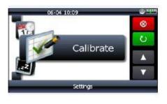
Carefully press and briefly hold stijus on the center of the target, Repeat at the target moves around the screen.
