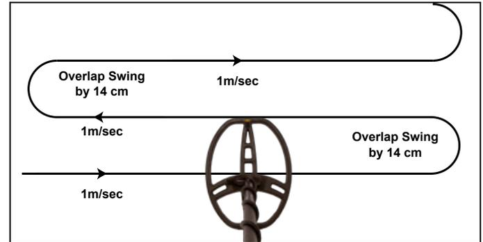
In order to fully search an area, overlap the swings of your searchcoil by half the length of the coil (about 14 cm). Sweep the searchcoil in a straight line or with a slight arc at a sweep speed of about 1m/sec.
