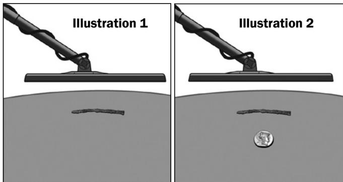
Iron targets, such as the nail shown above, can sometimes mask a good target. If too much iron discrimination is applied, the good target can be missed. Read page 23 to learn how to apply the proper amount of iron discrimination to eliminate the nail shown in Illustration 1 and still detect the good target shown in Illustration 2.
