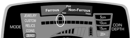
Use the DISCRIM buttons to position the Target ID Cursor above the pixel you wish to eliminate (see *above illustration*). Use the Accept/Reject pushbutton (✓/X) to delete this pixel from the Lower Scale (see *below*). This item is now rejected.
