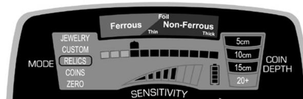
In Illustration 2, one of the same iron nails is laying above a good coin target. Since three pixels of ferrous have been notched out, the nail by itself would not be detected; however, the two objects have a **combined conductivity** of four pixels.
