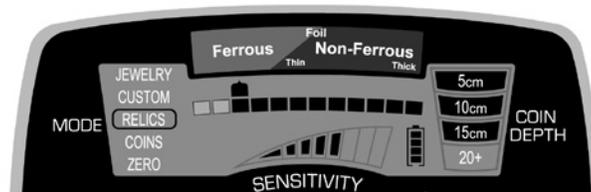
In the illustration above, the *EuroACE* is operating in RELICS Mode, with two pixels of iron discriminated. The nail seen in Illustration 1 (on page 22) registers above the third pixel. These ferrous targets can be eliminated from detection by using the Accept/Reject pushbutton (✓/X) to turn off the third pixel from the left.
