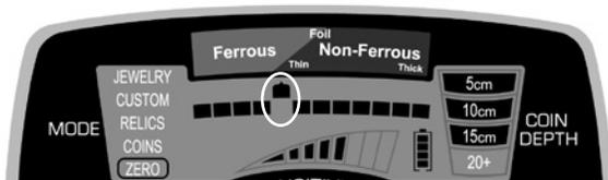
The second method of modifying the Notch Discrimination pattern involves the use of only the Accept/Reject pushbuttons. When an unwanted metal target is audibly detected while hunting, simply push the Accept/Reject button to create a notch where the Target ID Cursor has signaled the presence of the trash. The next time the *EuroACE* encounters the same trash item, it will not produce an audible signal.
