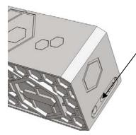
Power Up the speaker by pressing the ON/OFF kno on the right downside. For Off just press it again.
