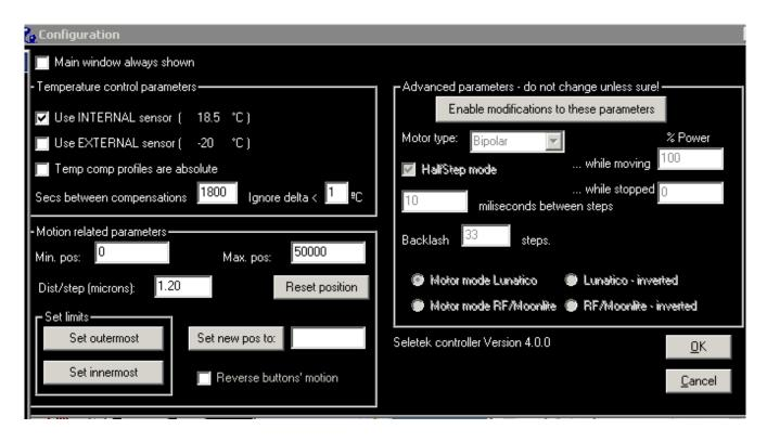
Proceed with the Rotator (Exp port) and enter the parameters. At "A" you have to enter the step count of the motor (written on the back of it, 200 or 400). At "B" set the voltage in percentage of the supply to protect the driver from overheating. With 12V enter 70%, with 15V
