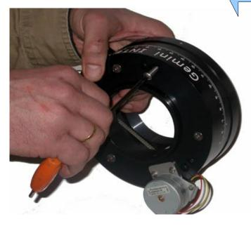
Now you can insert the 3 pc M6 mounting screws with a 4mm allen key into the larger openings and all the way down till you can see them come out at the bottom.
