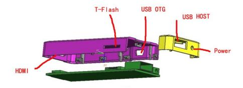
HDMI: mini HDMI connection - use the cable provided to connect the PC to a TV or monitor for Audio and Visual output
