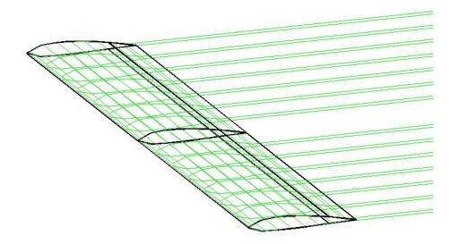
After setting those parameters, you create the geometry: the length of the following vectors is the number of the lifting surface segments you create. Each element is a surface section: if you want your surface to have 57 (hope you don't) segments and the 56<sup>th</sup> to have an aileron, you add 57 elements in the following vectors and put FCR zero to any of them, and the right flap chord ratio on the 56<sup>th</sup> element of the vector!
