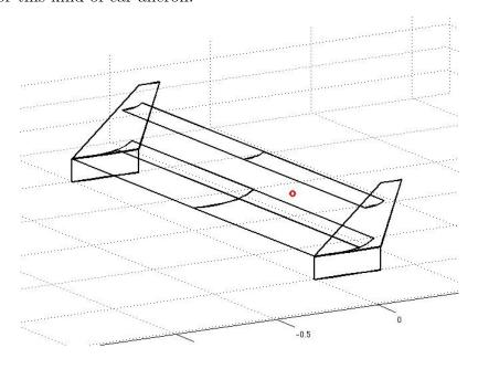
surfs().No is the number of panels chordwise. It is the same for every lifting surface section, but of course it can differ from one lifting surface to another!
