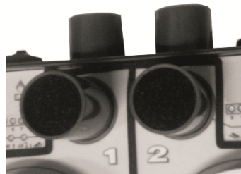
Figure 4-3: Filter at inlet of system
