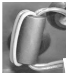
Figure 3-2: Ferrite core and battery supply wiring
