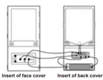
When user want to change battery, must separate the face cover and back cover by knife carefully, open it and replace the old battery by new and the same standard battery in battery house, then close the face cover and back cover. Be careful not to break the wire.
