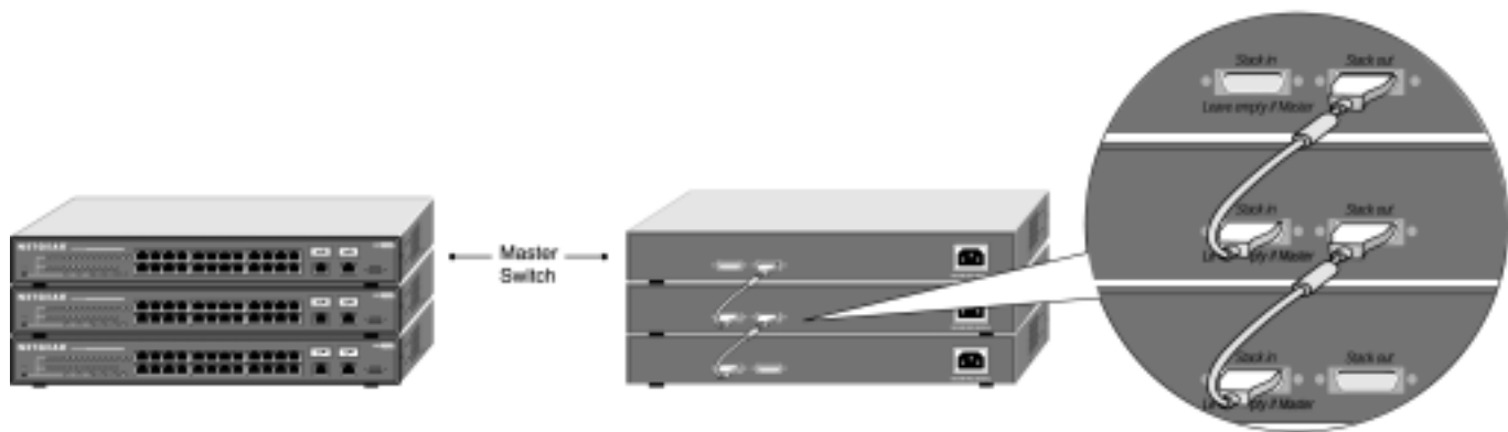
Figure 3-5. Cabling Three FSM726S Stacked Switches
