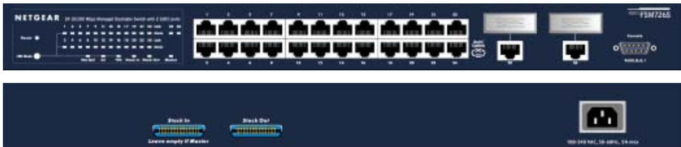
Figure 2-1. Front and Rear Panel of the FSM726S Managed Stackable Switch
