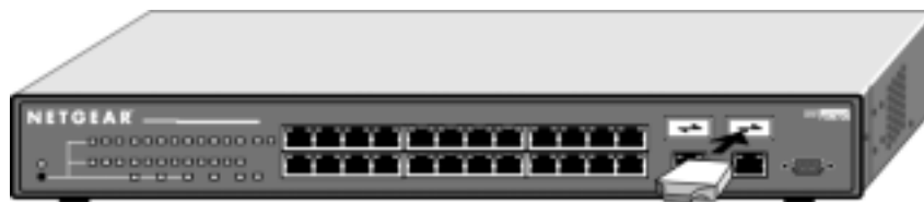
Figure 3-3. Installing a Gigabit Ethernet Module into an FSM726S
