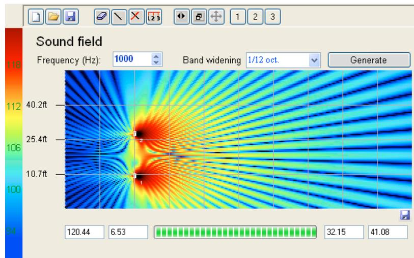
Experiment with different frequencies. Click generate after selecting a new frequency to plot. 1/12<sup>th</sup> of an octave is the highest frequency resolution, possible, but you can also choose to display the average of the full 10 octave response, shown below.
