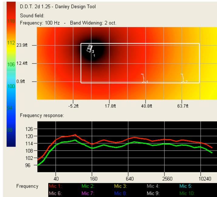
Moving the Sub to the ceiling immediately makes the response at the two mics virtually identical except for the level loss due to the difference in distance between the mics and speaker cluster. Again, feel free to experiment with different settings of the crossover, levels and delay. You may be able to improve on this design! Here is my best effort!
