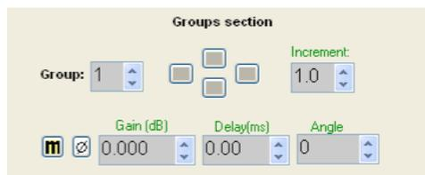
The group can be muted, the polarity of the entire group flipped, the gain can be changed, delay added and the angle of the speakers in the group adjusted. Using the 4 boxes between the *group select* and the *increment* boxes moves the entire group around, each click moving the group by the increment selected in the *increment* box.
