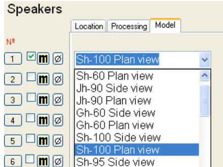
Selecting the box indicated by the arrow, makes the chosen speaker active. The *M* button next to it, is a *Mute* button, which leaves the speaker on the screen, but mutes the output. The phase button flips the polarity of the speaker.
