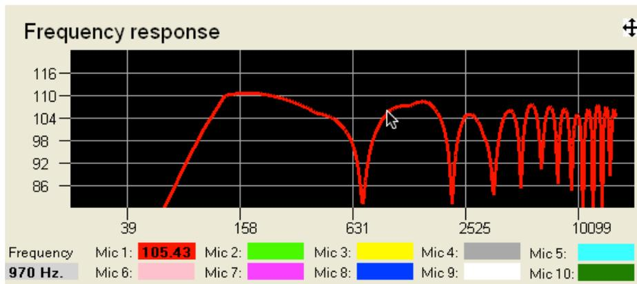
This is the frequency response of the system at that point in space. There is clearly a lot of “comb filtering” due to the arrival times from the two speakers. To confirm this you could simply mute one of the speakers. You will see the response immediately flatten out.
