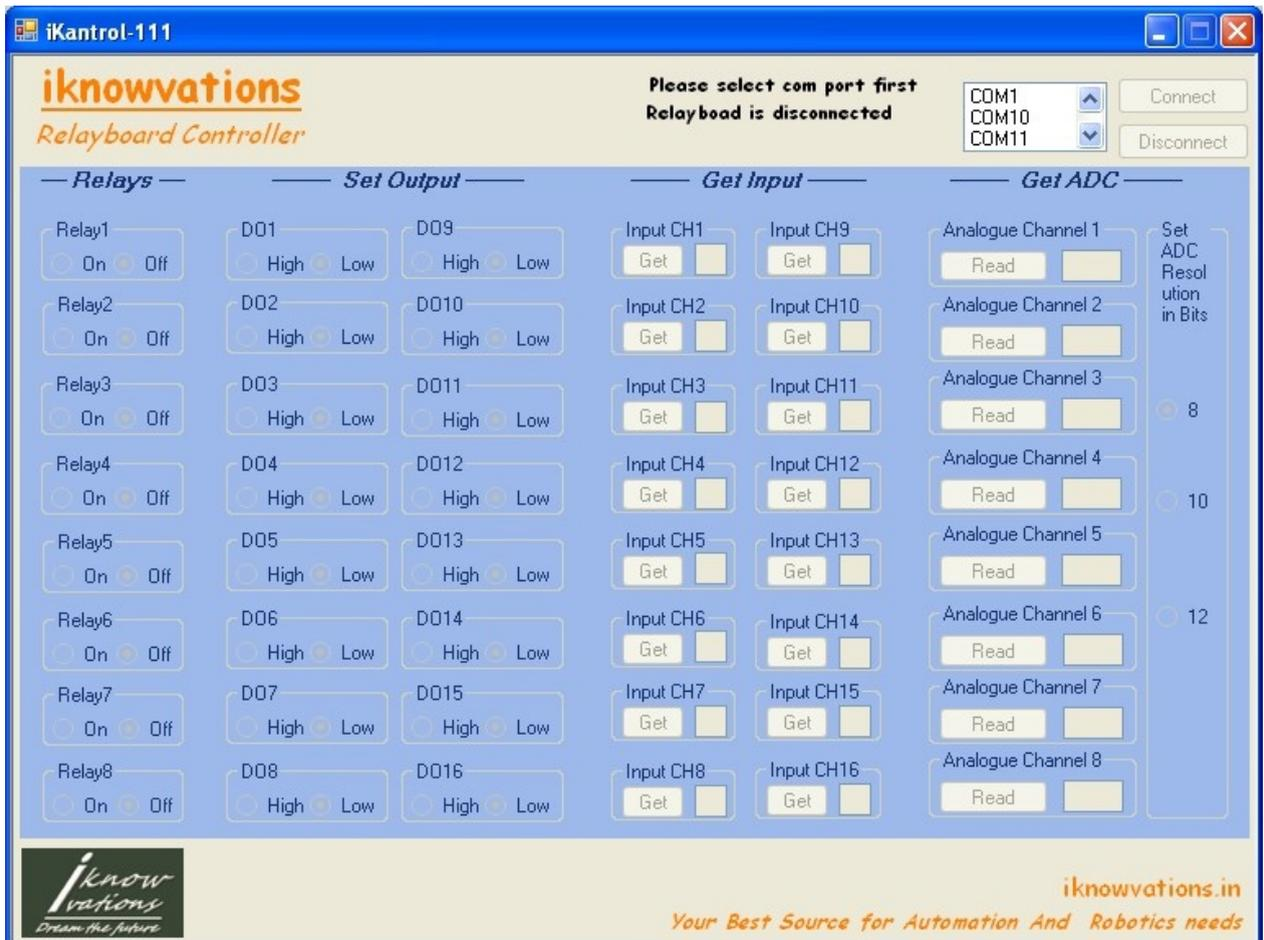
Select the com port to which you have connected the card U452 from available com port list. Press connect button. If the card is connected you will get next screen with all the buttons enabled in blue panel.
