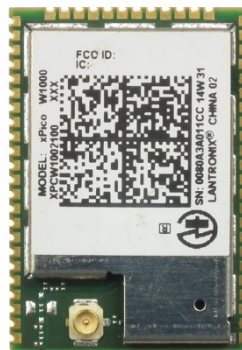
Figure 2: xPico W1003 (XPC W1003) Embedded Device Server
