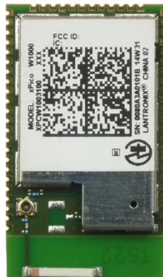
Figure 2: xPico W1003 (XPC W1003) Embedded Device Server
