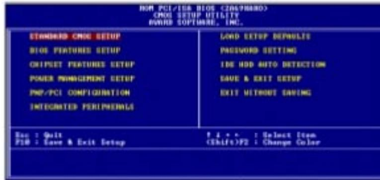
Figure 5-1: Setup program initial screen
