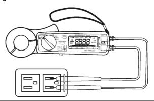
**WARNING:** Maximum input for DC V is 600, and for AC V is 600. Do not attempt to take any voltage measurement that exceeds the limits. Exceeding the limits could cause electrical shock and damage to the clamp meter.
