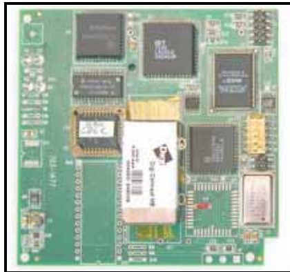
Figure 55: XMT BACNet/IP Option Card
