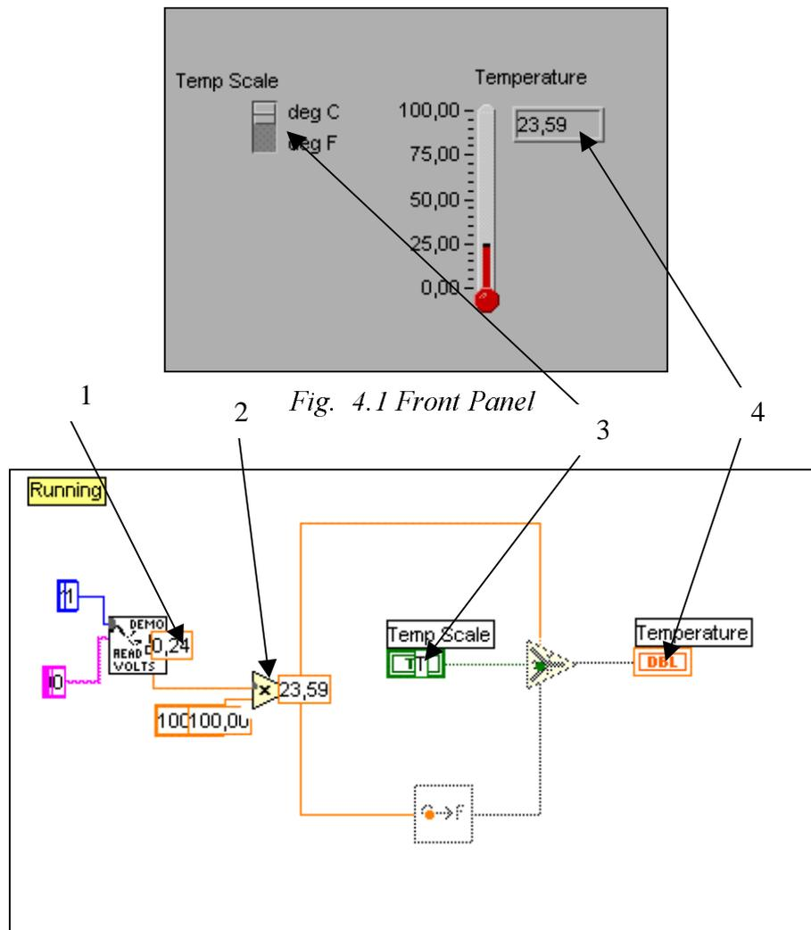
Fig. 4.2 Dataflow Diagram
