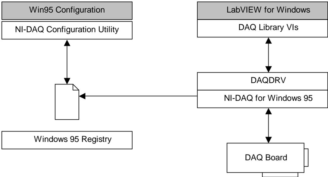
Fig. 3.1 Data Acquisition Model
