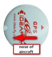
GPS /compass is sensitive to magnetic interfence, should be far away from any electronic devices. If your own mounting rod. make sure it is NOT magnetic.
