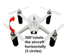
Quickly flip CH5 switch from manual mode to GPS mode and back to manual mode for more than 3 times. LED indicator will be turn on solid green
