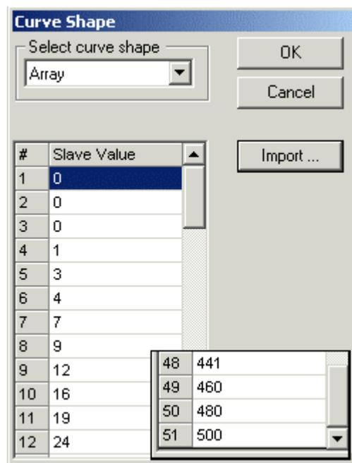
**Figure 39: Example of Curve Shape Menu with Completed Array Table**
