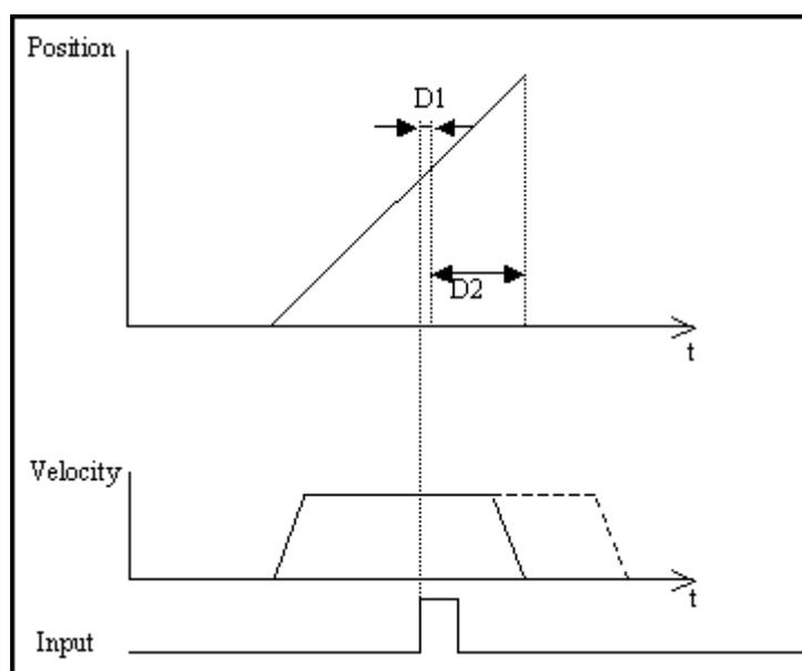
**Figure 50: Illustration of Motion Terminated by Registration**
