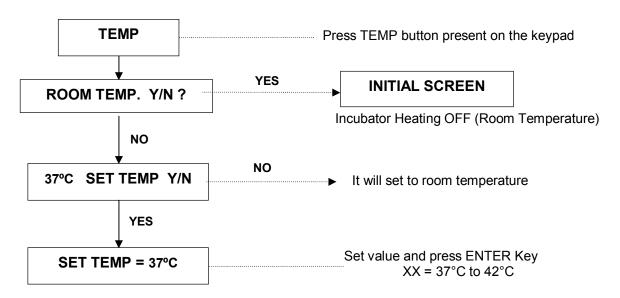
**NOTE**: By Default condition incubator heating is off, Instrument will show Room Temperature
