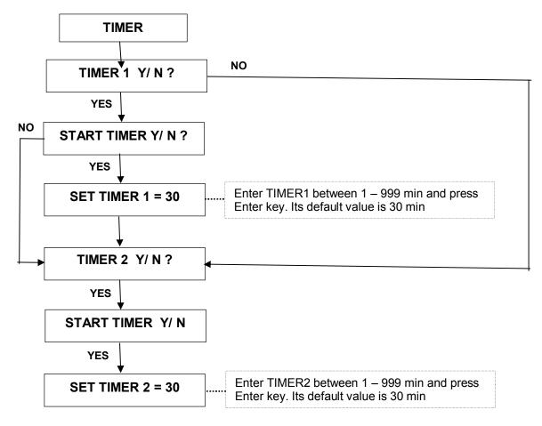
After selecting Timer1 and Timer2, LED glows of the respective Timer. On completion LED gets OFF and the buzzer beeps in order to indicate that the Timer has reached its set value. Now select Enter key to stop the buzzer.
