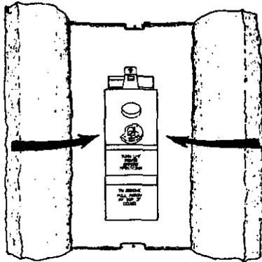
19. The adjustment dial has a "D" shaped opening that matches a "D" shaped shaft on the thermostat. Align the opening in the dial to the shaft and gently push the dial onto the shaft.
