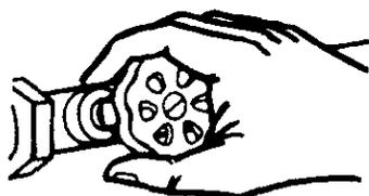
3. Attach a hose to the water heater drain valve and put the other end in a floor drain or outdoors. Open the water heater drain valve. Open a nearby hot water faucet which will relieve pressure in the water heater and speed draining.
