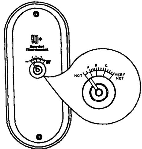
**LOWER THERMOSTAT ADJUSTABLE THROUGH LOWER ACCESS PANEL**
