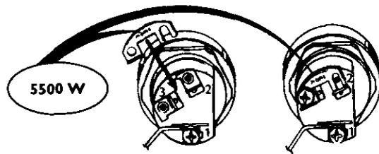
8. The wire removed from terminal 2 has a looped end. It must remain looped and now be placed (as shown) on top of the buss bar, over the opening of terminal 2, and secured using the remaining screw.
