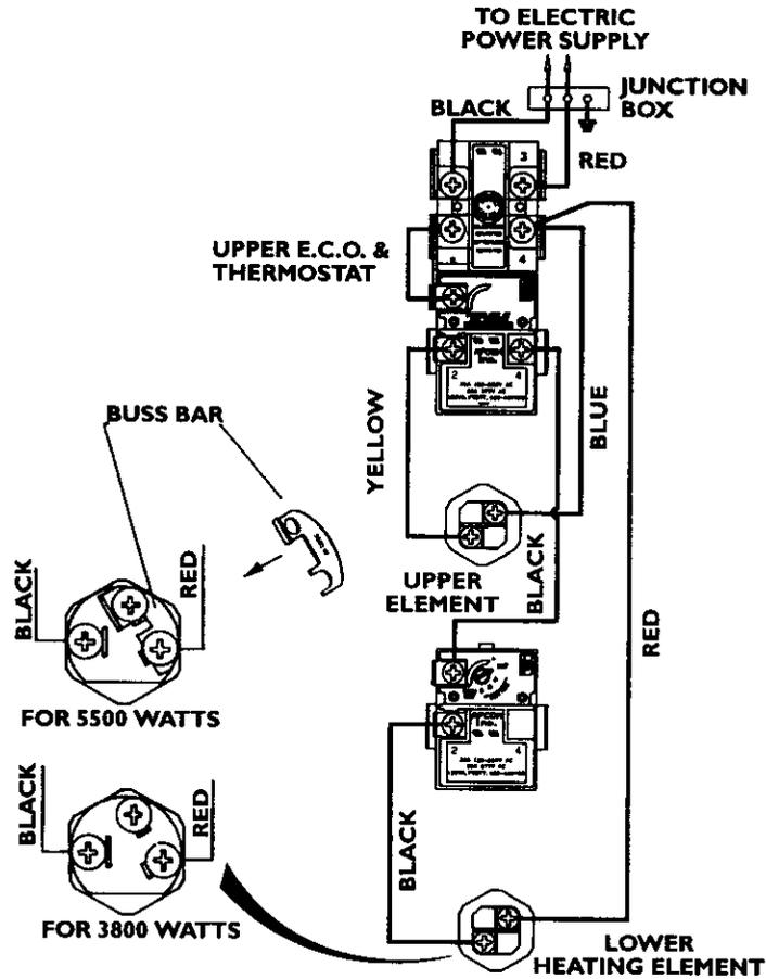
WIRING FOR 3 WIRE LEAD WATER HEATERS
