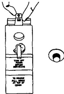
20. Turn "ON" electric power to water heater.
