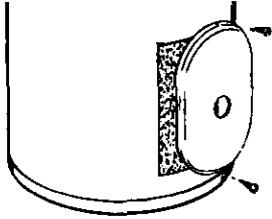
3. Remove the adjustment dial from the thermostat by gently pulling it directly away from the thermostat.
