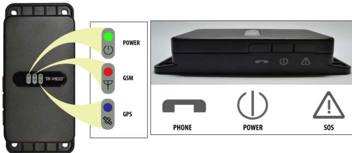
Figure 3 - T23 FLEET Control Panel
