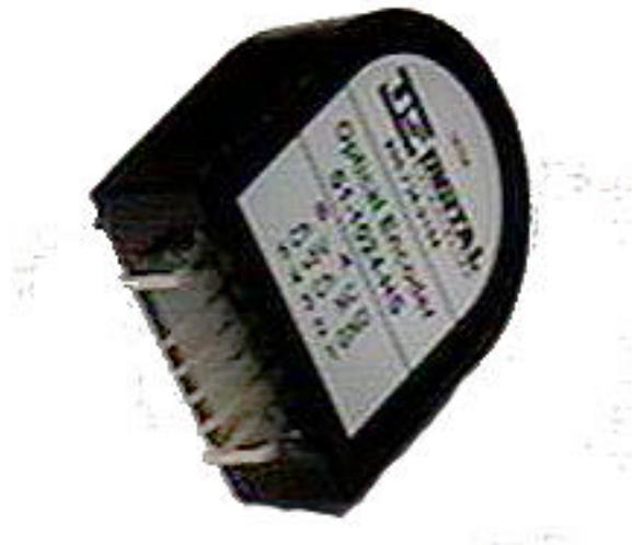
Figure 4.2 – A typical small quadrature encoder
