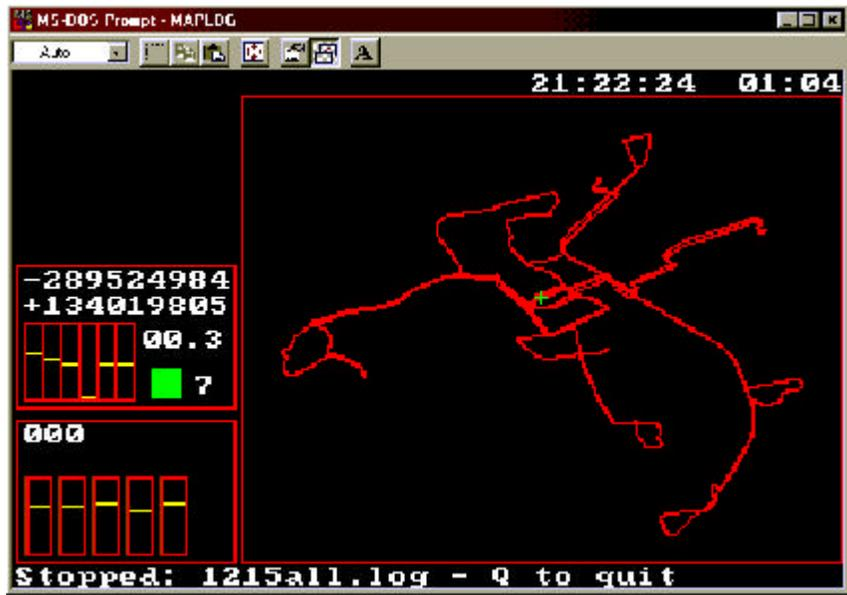
Figure 6.5 – Maplog data acquisition program showing plot of GPS data
