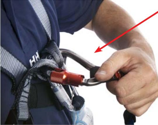
The Runner/Slider attachment in the harness always has to be executed with the Release-Strap attached on top of the Runner/Slider connector.
