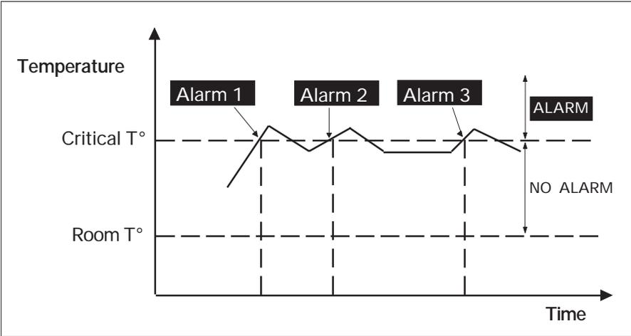
In the second case, the system monitors the difference between the room and outdoor temperatures. When this difference is greater than the offset, an alarm is set off.
