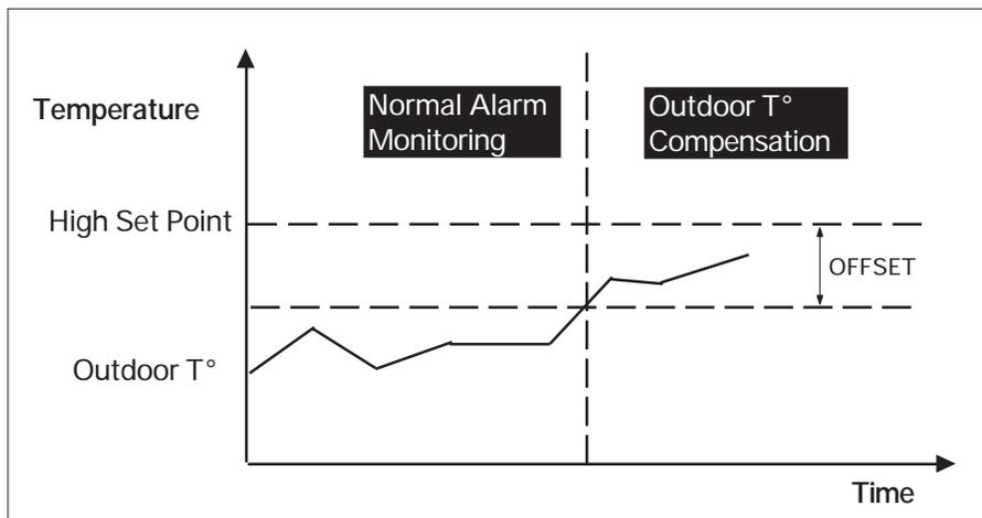
When outdoor temperature compensation is in effect, the system monitors (i) the room temperature with respect to the critical temperature (this check has the highest priority); (ii) the room temperature with respect to the outdoor temperature. The figure below illustrates the first case:
