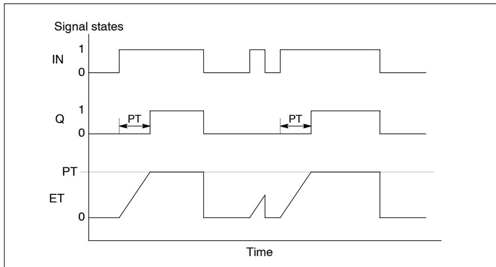
Figure 5-21 Timing Diagram for On-Delay Timer (TON)
