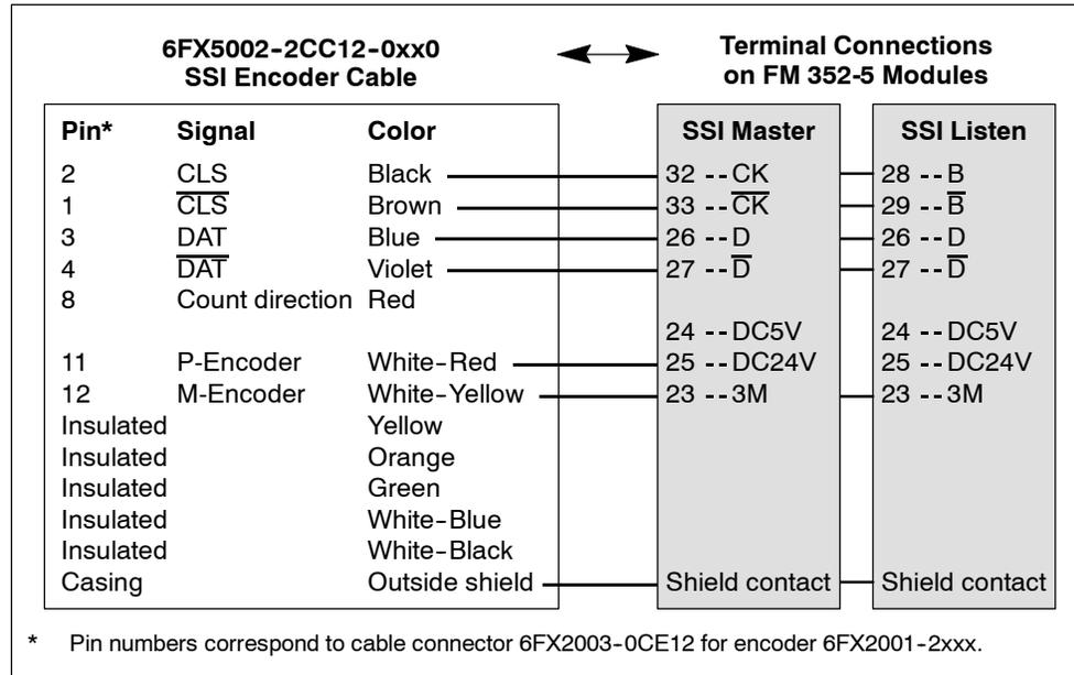
Figure 3-4 Wire Connections for SSI Encoder from SSI Encoder Cable
