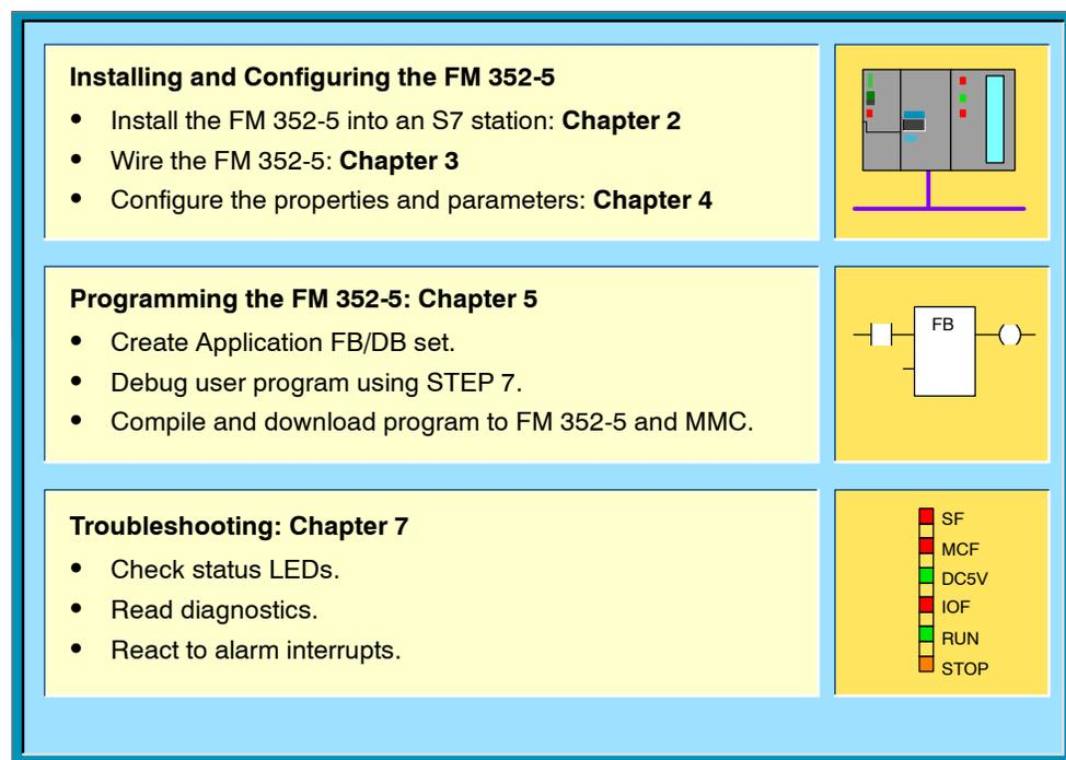
Figure 1-5 Basic Tasks to Set Up and Operate the FM 352-5
