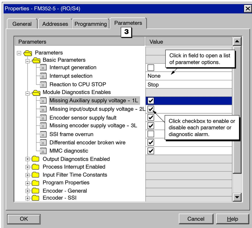
Figure 4-5 FM 352-5 Properties Dialog, Parameters Tab
