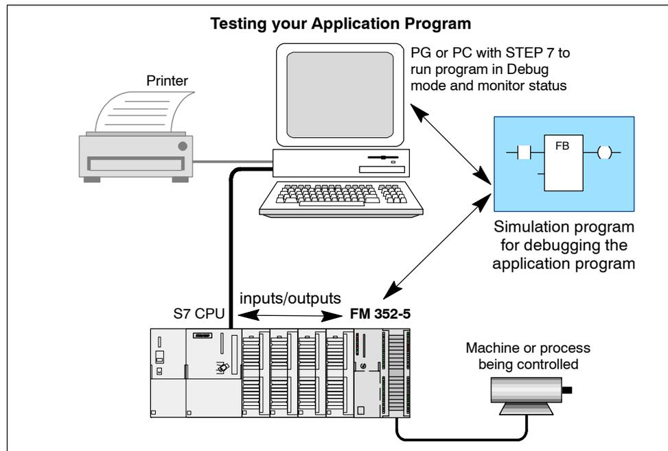
Figure 1-4 System Configuration for Debugging your Program
