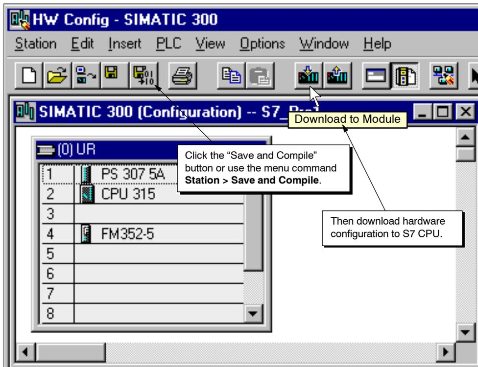
Figure 4-6 Saving and Compiling the Hardware Configuration
