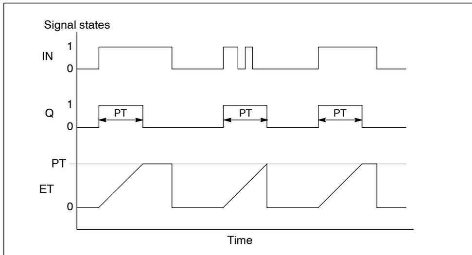
Figure 5-20 Timing Diagram for Pulse Timer (TP)
