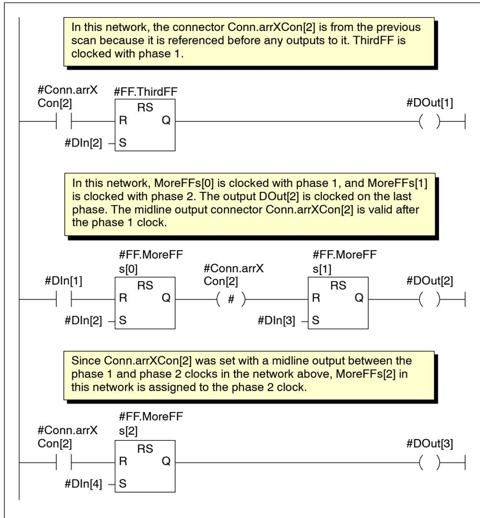
Figure 5-11 Examples of Multi-phase Clocking of Retentive Elements
