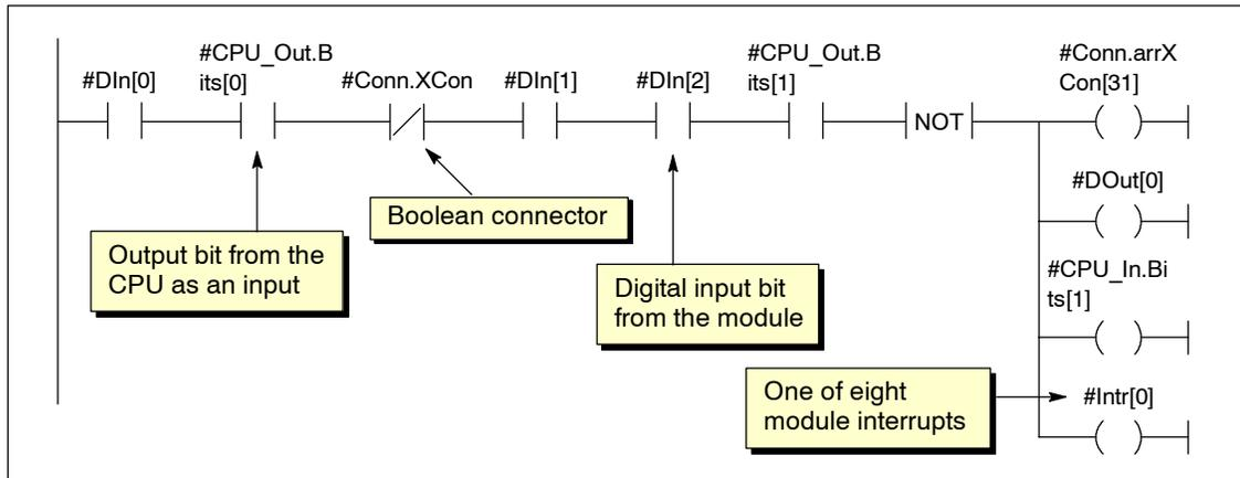
Figure 5-5 Input and Output Operands Allowed by FM 352-5
