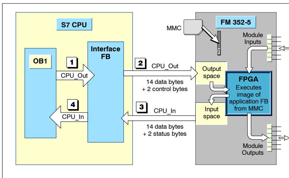
Figure 5-16 Data Exchange in Normal Mode
