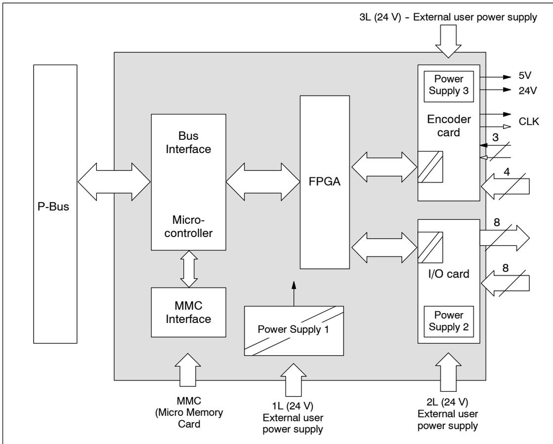
Figure A-1 Functional Block Diagram of the FM 352-5 Module
