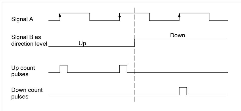
Figure 6-6 Pulse & Direction Counting
