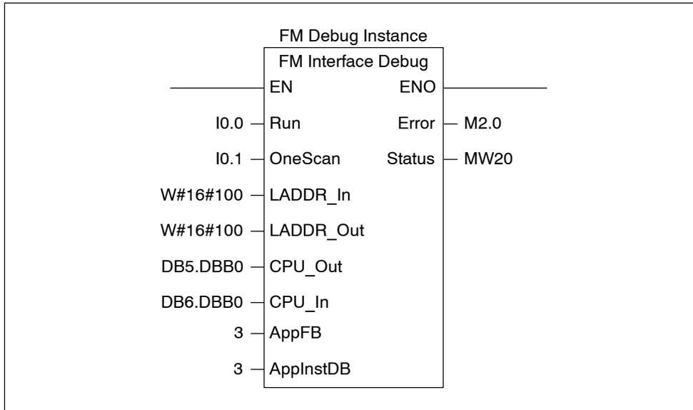
Figure 5-13 Interface FB for Debug Mode Execution
