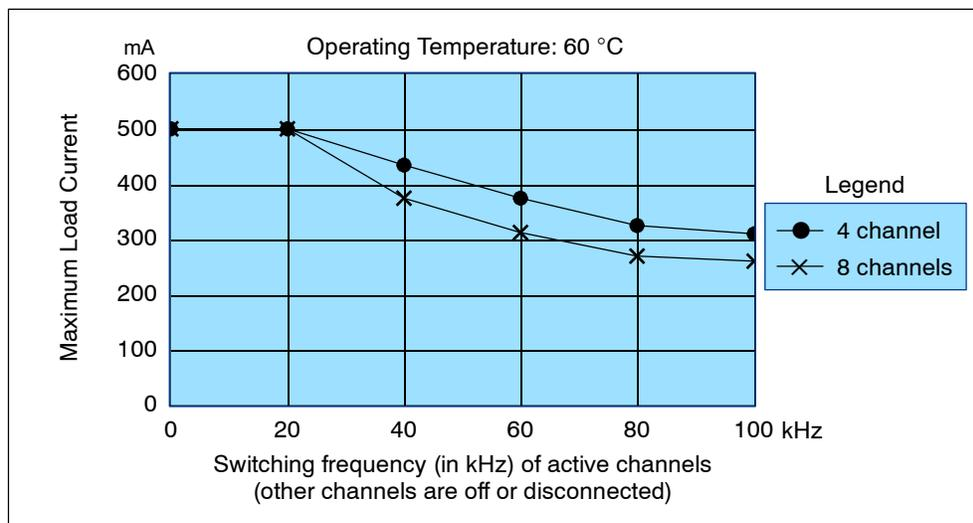
Figure A-3 Switching Frequency vs. Maximum Output Current at 60 °C
