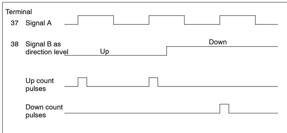
Figure 6-5 Signals of a 24 V Pulse Encoder with Direction Level
