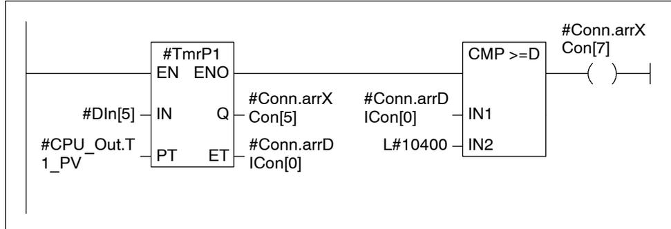
Figure 5-6 Example of a 32-Bit Pulse Timer from the Library FBs
