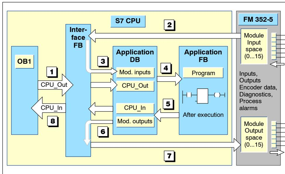
Figure 5-14 Data Exchange in Debug Mode
