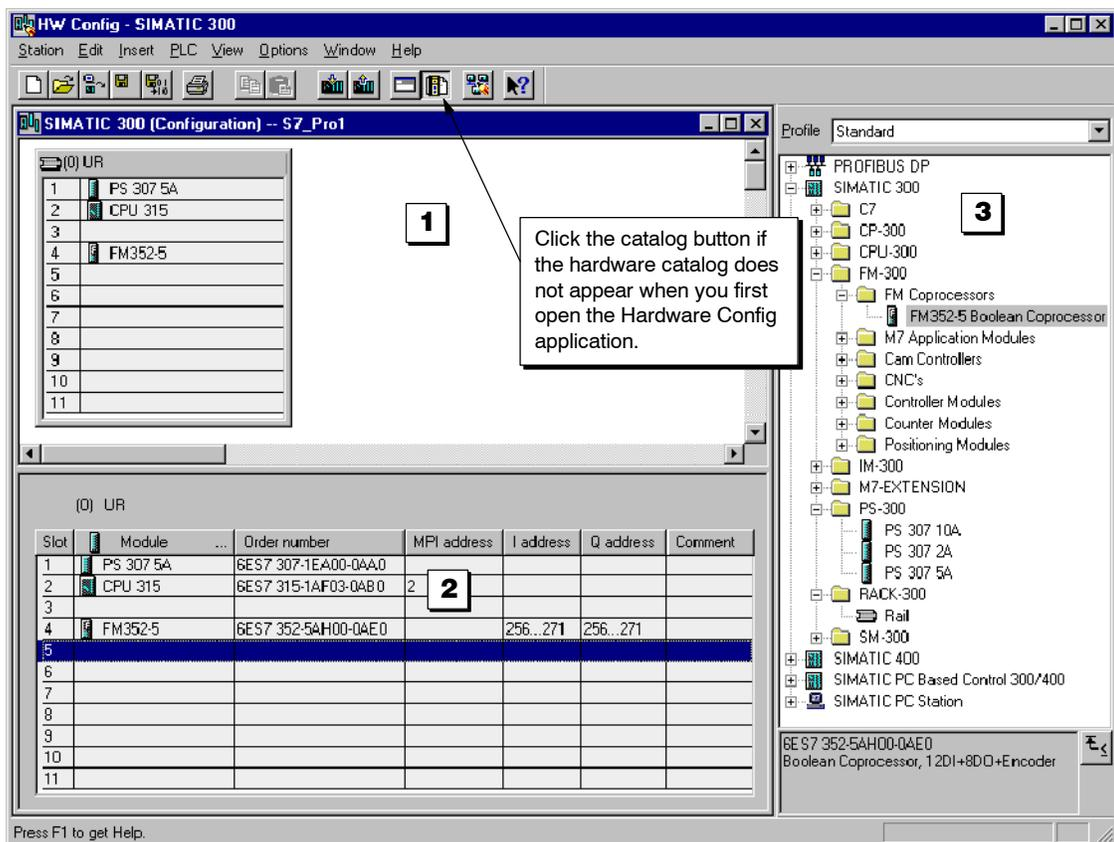
Figure 4-2 Hardware Configuration Window
