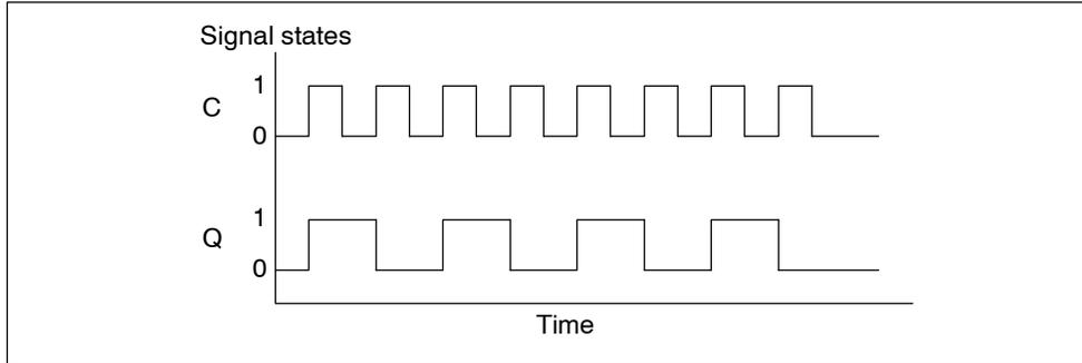
Figure 5-19 Timing Diagram for Binary Scaler (BiScale)
