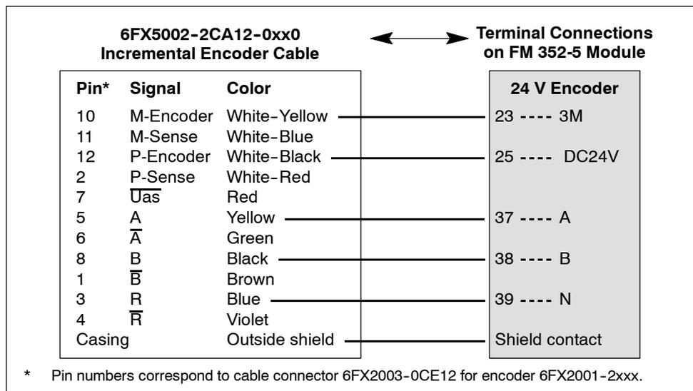
Figure 3-3 Wire Connections for 24 V Encoder from Incremental Encoder Cable
