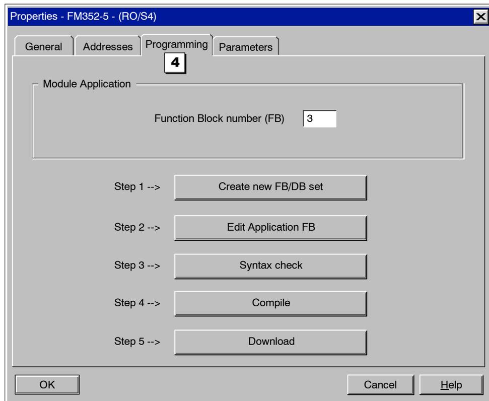
Figure 4-7 FM 352-5 Properties Dialog, Programming Tab
