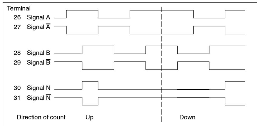
Figure 6-4 Signals of the Differential Incremental Encoder
