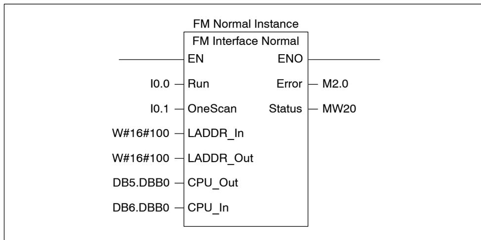
Figure 5-15 Interface FB for Normal Mode Execution
