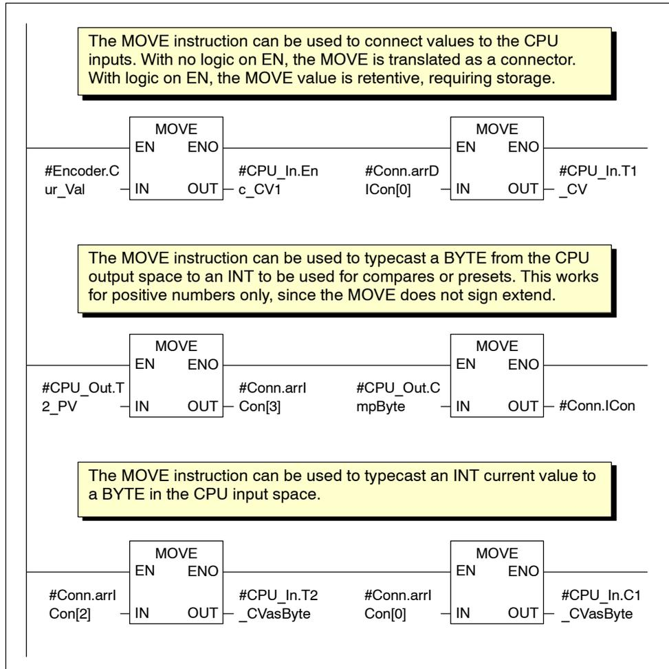
Figure 5-8 Examples of MOVE Instruction with Typecasting
