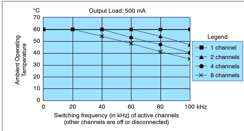
Figure A-2 Switching Frequency vs. Ambient Temperature at 500 mA Output Load
