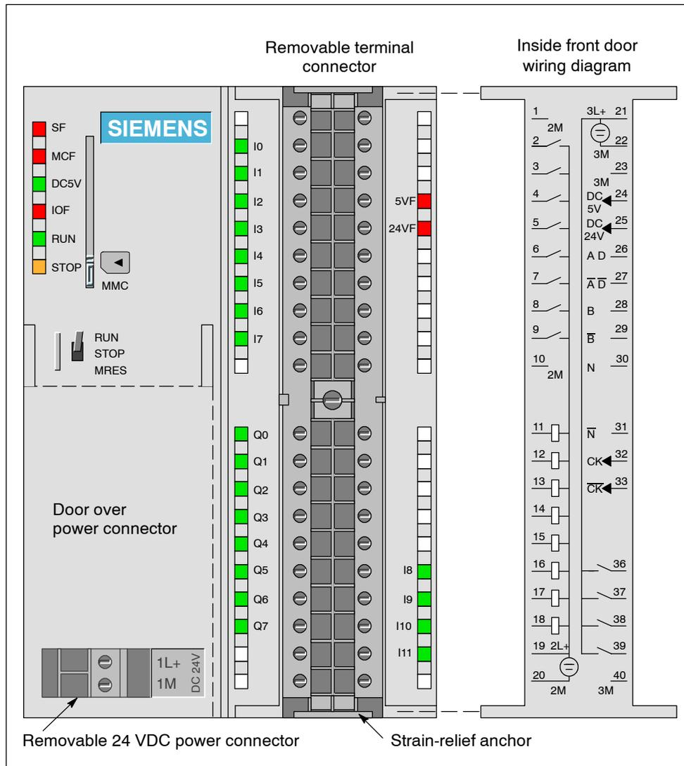
Figure 3-1 Front Terminal Connector of the FM 352-5
