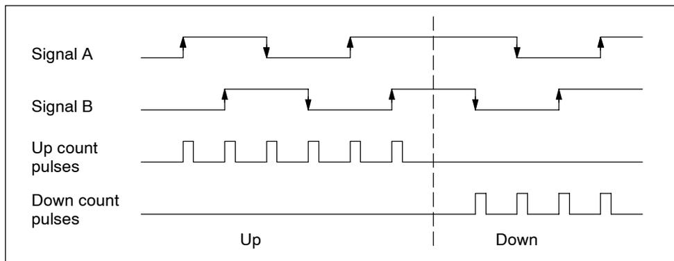
Figure 6-9 Quadruple Evaluation
