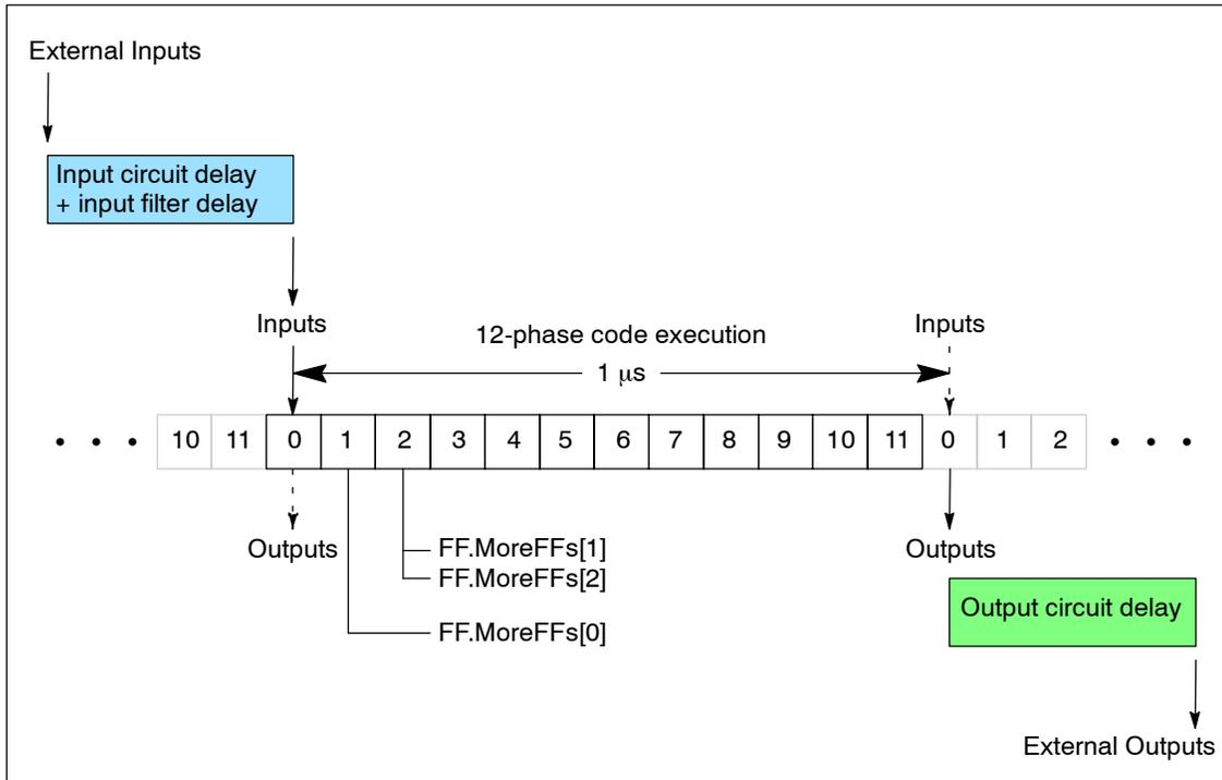
Figure 5-12 Multi-Phase Clocking and I/O Timeline
