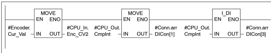
Figure 5-9 Example of MOVE and I\_DI Instructions for Typecasting
