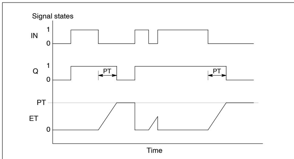
Figure 5-22 Timing Diagram for Off-Delay Timer (TOF)
