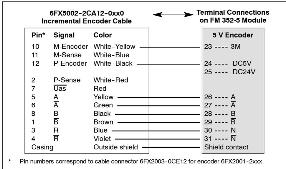
Figure 3-2 Wire Connections for 5 V Encoder from Incremental Encoder Cable
