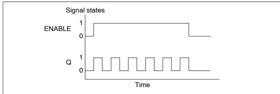
Figure 5-23 Timing Diagram for Clock Pulse Generator (CP\_Gen)
