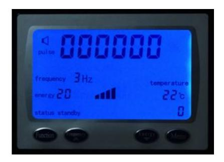
The STAND-BY MODE is used for safely setting the TREATMENT PARAMETERS, such as FREQUENCY, ENERGY LEVEL. In STAND-BY MODE the HAND-GUN PIECE WILL NOT FIRE.
