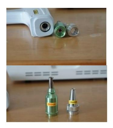
Carefully unscrew the **1064nm GUN TIP** and store in a location where it will not be dropped or knocked-over.
