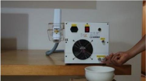
( BEFORE filling the UNIT with water, remove the AC POWER CORD from RECEPTOR, and place a small container under the OVERFLOW CAP so that the excess water can be emptied from the UNIT and disposed of properly.)
