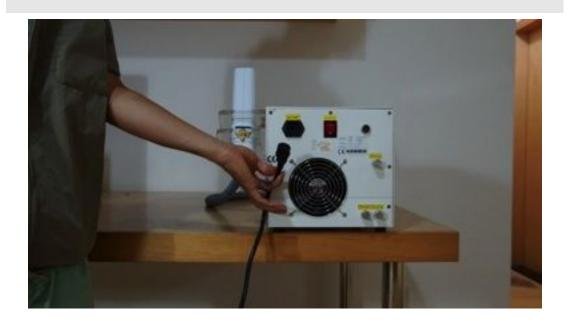
**2)** FOOT-PEDAL SWITCH: Plug the FOOT-PEDAL into its RECEPTOR at the REAR of UNIT. This plug includes a SAFETY LOCK-SCREW which should be tightened securely.
