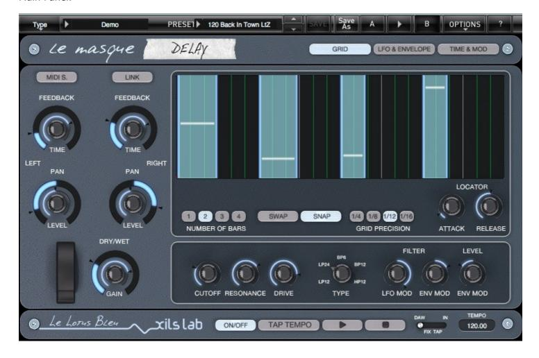
You'll find on the main Panel the following areas: The Delay Settings area, the Filter Settings and Live Modulation Area, The TAP bar with all the clock and sync options, the Preset Management bar, and finally The Grid itself with the Mask(s)
