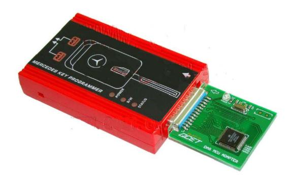
**2.**Open the software. You need click **[Check Port]** first, software will remind you switch to M1 mode, the red indicator light should light, and then click **[OK]**. It will find out the right COM-PORT automatically. Please note that: COM-PORT must be in "COM1-COM4" you can get more information at previous page, "PART TWO: Port Setting". After that, the software will show the correct port that you are using now. As below shows:
