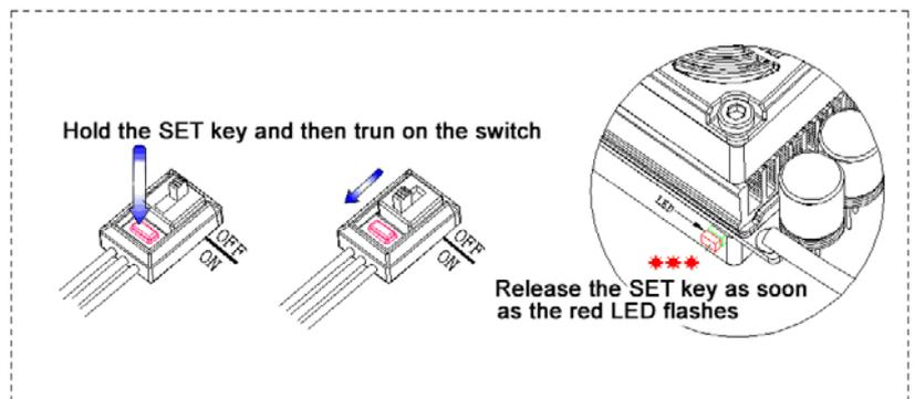
**Note4:** If you don't release the “SET” key after the red LED begins to flash, the ESC will enter the program mode, in such a case, please switch off the ESC and re-calibrate the throttle range again from step A.
