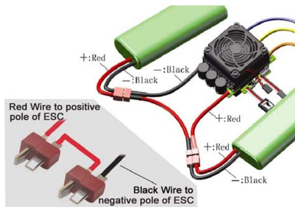
**Note3:** There is a small female connector that coming out from the “FAN” socket, this is used for connecting with the cooling fan of the brushless motor.
