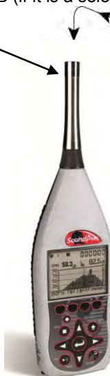
Figure 5-2: Attaching calibrator to SoundPro
