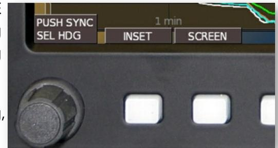
To immediately set the heading bug to the present heading, simply push the left knob to “sync” it.
