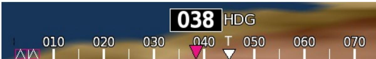
*This aircraft has flown off course to the right. The heading bug and the GPS waypoint bearing marker are both beyond range of the tape, so they are hollow and appear to be “stuck” at the edge of the heading tape. The pilot can get back on course by turning left, toward the heading bug and GPS waypoint bearing.*
