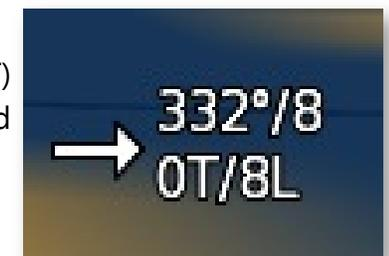
**NOTE:** If insufficient data exists for calculation of winds, the wind information is not displayed. Accurate winds require accurate magnetic heading and airspeed data, which are enhanced by performing proper calibration of magnetometer and pitot/static systems as detailed in the HXr Installation Manual (also the HX User Manual, Rev. C, Section 9).
