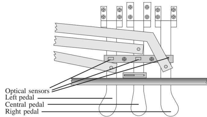
To access the optical sensor on the pedals board unscrew the two screws and turn it up.
