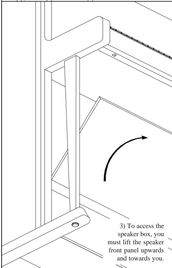
3) To access the speaker box, you must lift the speaker front panel upwards and towards you.
