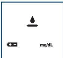
The **+ -** symbol appears on the display with the unit of measure. The power is getting low. It is time to change your battery.
