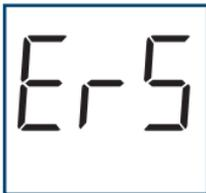
Error message that indicates that the meter has detected a problem with the test strip. Possible causes are test strip damage or an incompletely filled confirmation window.
