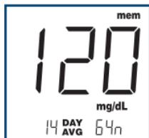
Average of results from the last 14 days (64n means that 64 tests were performed within the period). The 30-day average appears with a 30 before the DAY AVG on the screen.
