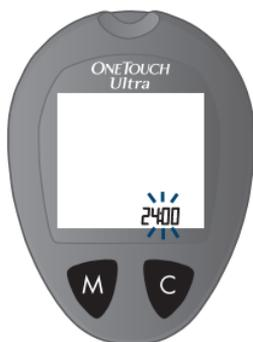
Press and release the **C** button to choose between AM/PM and 24-hour formats.
