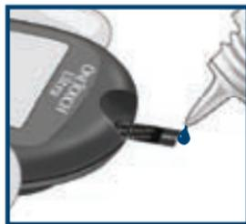
Touch and hold a drop of control solution where the narrow channel meets the TOP EDGE of the test strip.
