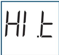
The meter has detected that the temperature is above the system operating range. **Do Not** perform a test until the meter and test strips reach a temperature within the operating range of 43–111°F (6–44°C).
