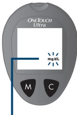
Press and release the **C** button until mg/dL appears on the display.
