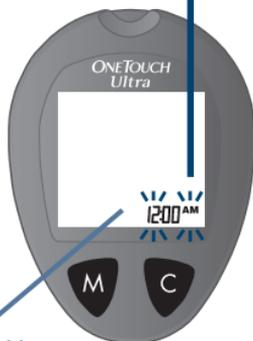
Flashing indicates setting can be changed
