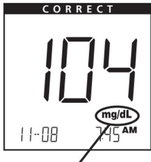
If your meter is set to the correct unit of measure, “mg/dL” will appear on the display. Your test result will not include a decimal point (Fig. 1). **Do Not** change this setting – this is the correct unit of measure for the United States.
