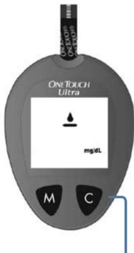
Press and release the **C** button so **ctl** appears on the display.
