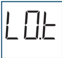
The meter has detected that the temperature is below the system operating range. **Do Not** perform a test until the meter and test strips reach a temperature within the operating range of 43–111°F (6–44°C).
