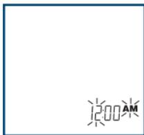
Flashing time means the meter has lost power and entered the setting mode.
