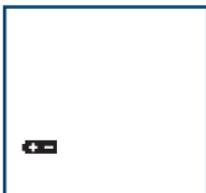
The **+ -** symbol appears on the display by itself. The power is too low to perform a test.
