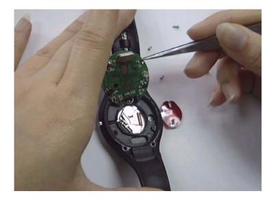
4 •Remove the red insulator and replace the battery, screw back the CBA first and then the case back
