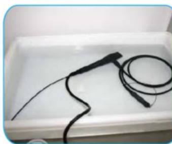
If the needle position remains steady. Immerse the entire scope in water and observe for 30 seconds. Angulate the distal bending section up and down while the Endoscope is immersed. The absence of air bubbles confirms the scope is air tight. Remove from water and open the leak tester's valve. Ensure the needle on the pressure gauge fails to zero and disconnect the leak tester from the endoscope.
