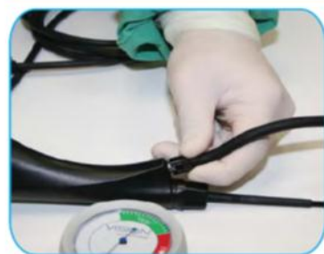
Connect the leak tester to the endoscope's EtO/vent valve. Push down and rotate the leak tester connector clockwise until it is secured.
