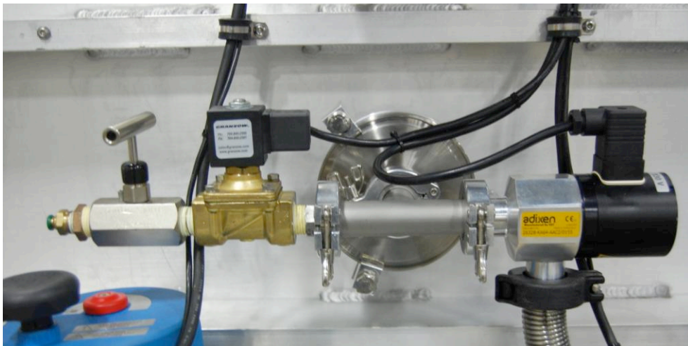
Figure 4 – Detail View of Vacuum Manifold
