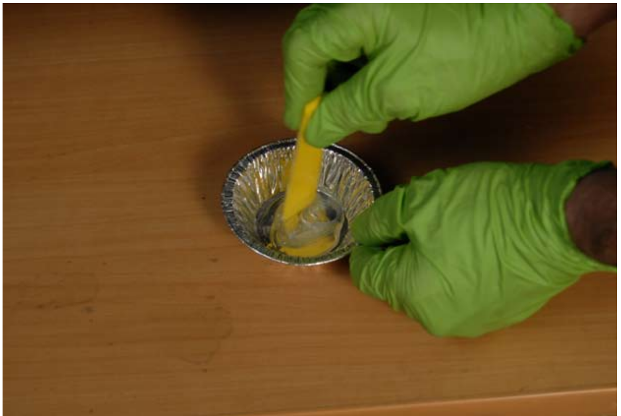
▲ Mix epoxy resin, following manufacturer's instructions.
