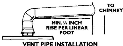
There must be a minimum of 6" clearance between single wall vent pipe and any combustible material. Fill and seal any clearance between single wall vent pipe and combustible material with mortar mix, cement, or other noncombustible substance. For other than single wall, follow vent pipe manufacturer's clearance specifications. To insure a tight fit of the vent pipe in a brick chimney, seal around the vent pipe with mortar mix cement.
