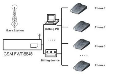
The sketch for connecting to Billing device or Computer charging system
