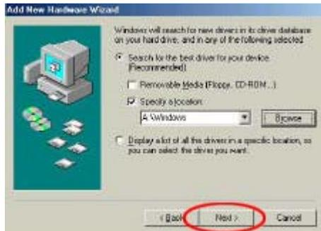
The driver will be NEC PCI to USB Enhanced Host Controller” When you see the screen, click “Next.”
