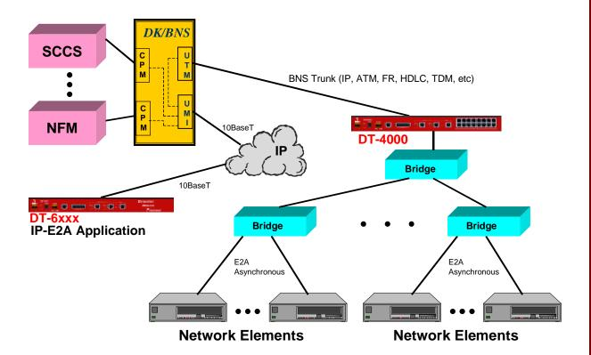
In the diagram above, the **DT-6xxx** is executing the **IP-E2A** application that interfaces to the SCCS and NFM operations system without changes. As far as these operations systems are concerned, they are communicating via a Datakit E2A port. This allows a smooth and effective migration of these components.
