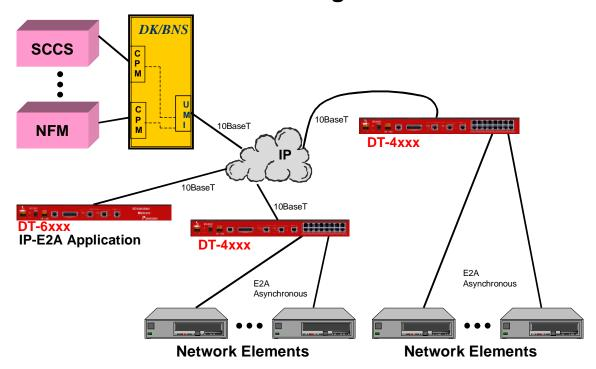
There may be a situation where an OS, such as NMA, provides support for E2A endpoints with dedicated hardware. The NMA OS also supports the virtual interface. However, should the dedicated hardware interface be desired, the deployment would be as follows:
