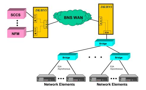
The operations system communicates with a central access point for a set of network element on a bridge network. This is a serial port an a BNS/Datakit E2A card, or it may be a direct interface on the host if there is no BNS/Datakit network present. The central access point is attached to one or more tiers of bridges to broadcast the message to multiple network elements. In some installations, these bridges are actually 202T data sets configured as a half duplex multi-drop distribution net.
