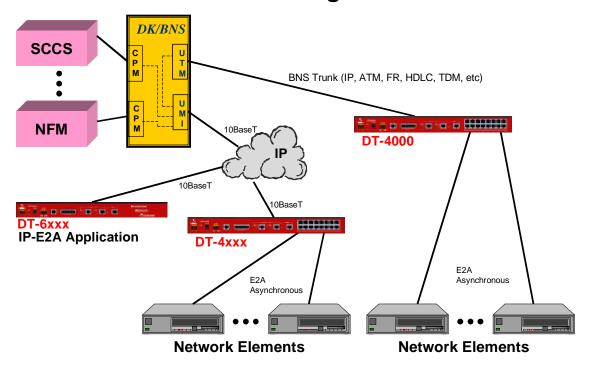
It should be noted that the functionality may traverse several network types. In the example shown above, both BNS and IP networks are being used. One DT-4000 is acting as a native BNS device, and another is acting as an IP native device. The interaction is completely seamless.
