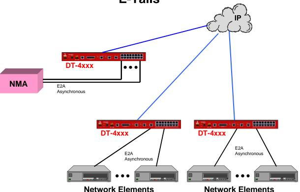
In the diagram above, the bridge exists at the OS head. Individual tail circuits are used to each network element. However, instead of a physical connection; the **DT-4xxx** is used for a logical connection using an embedded network. Each of these tail circuits (called E-Tails) can be individually diagnosed without affecting the others.
