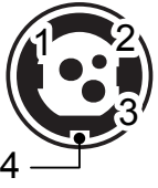
POWER SUPPLY Tripolar female connector
