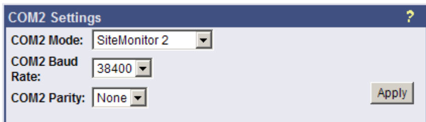
Figure 10: HTTP – COM2 settings to SiteMonitor 2
