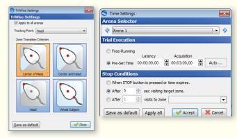
Specific settings provided for the accurate detection of animal behavior according to user-established criteria. The settings can be changed afterwards during analysis and the experiment replayed to obtain a new set of data.
